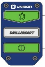
ONCE THE **MAGNET ON** BUTTON IS PRESSED THE MAGNET ON LIGHT WILL EITHER ILLUMINATE SOLID GREEN SHOWING ENOUGH ADHESION HAS BEEN ACHIEVED OR FLASH RED SHOWING NOT ENOUGH MAGNETIC ADHESION HAS BEEN ACHIEVED.
